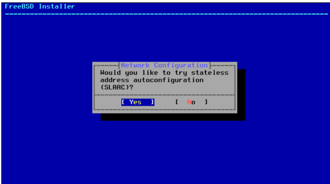
Figure 43. Choose IPv6 SLAAC Configuration
